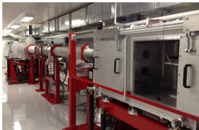
BELLA PW iP1: long focal length target chamber (right), laser diag. & e- spec. (left)
