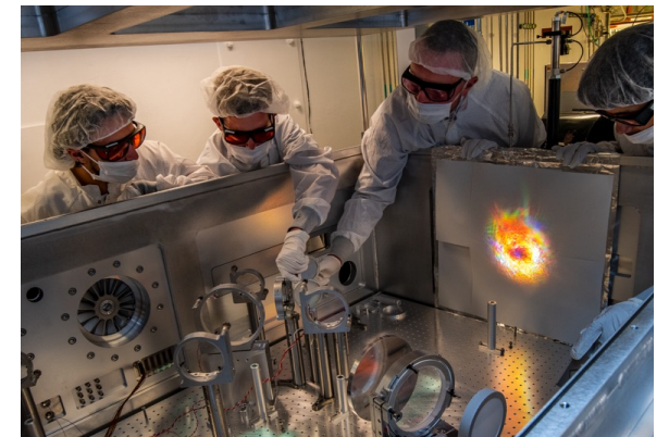
BELLA hundred-TW lasers: open chamber, flexible multi-beam work & photon sources
